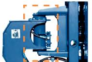
When a large load is applied to the basket, the basket rotation mechanism with hydraulic rotary actuator operates to release the load and decrease risk of damage.
