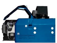
A gull-wing cover and swing-out engine base are utilized. The ease of maintenance and cleaning are improved.
