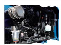
New Tier 4 engine reduces environmental burden. In addition, engine speed control in accordance with work load increases fuel efficiency.
