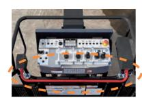
Bar-type touch switch is utilized. It can correspond to basket deformation and it is more reliable than previous wire-type switch.
